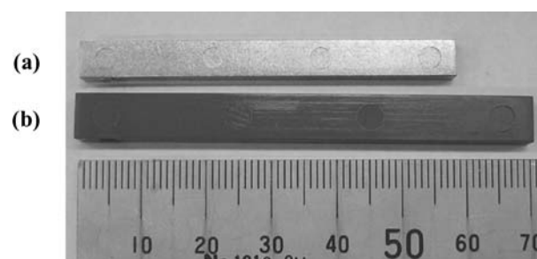
Figure 4 The shapes of (a) the final article after sintering and (b) green part prepared by feedstock 2 in Table II.
